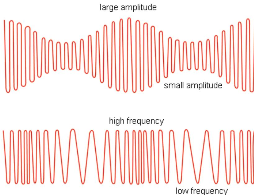
The upper trace is **amplitude modulated**. The amplitude changes from large to small to large again to copy the changes in the sound wave being carried by the radio wave. The frequency does not change.
