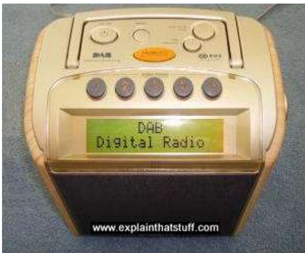
Photo: A typical Roberts DAB digital radio. The big orange button in the middle lets you pause a live radio broadcast and restart it later.
