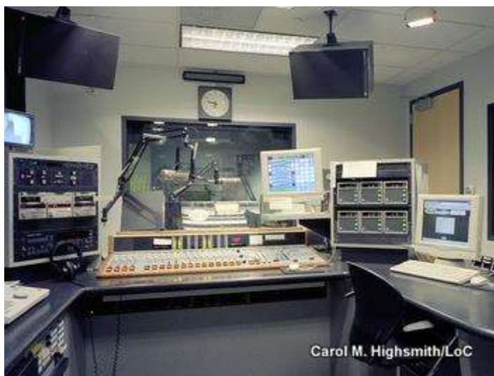
Photo: A radio studio is essentially a soundproof box that converts sounds into high-quality signals that can be broadcast using a transmitter. Credit: Photographs in the Carol M. Highsmith Archive , Library of Congress, Prints and Photographs Division.
